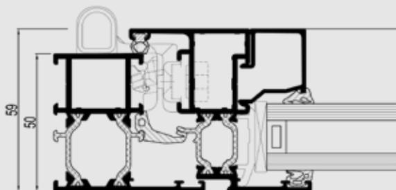
Eco System® 50 is a well-insulated system for windows and doors, that combines aesthetic design and energy efficiency with a moderate price. The system's HI+ variant achieves Uf values down to 1.6 W/m<sup>2</sup>K. The Uf of a frame/vent section with 86 mm visible width is 2.3 W/m<sup>2</sup>K.
